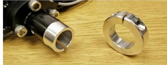
3. Collar shown in place. Rotate the collar so the split in the collar aligns with the split in the bottom of the handle shaft.
