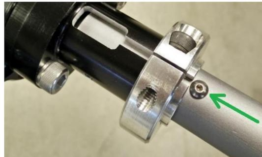
7. Tighten the socket cap screw in the clamping collar using the 3/16" Allen key.
