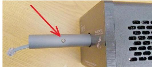
5. Check the orientation and plug the RJ12 connector into the jack inside the handle. The locking tab on the RJ12 connector should align with the slot in the handle collar.
